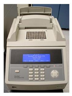
A thermal cycler heats and cools a DNA sample in order to perform the PCR. There are numerous thermal cyclers available from a variety of manufacturers. The instruments vary in the number of samples that can be handled, the size of reaction tube used, the speed of temperature change, and the cost.
